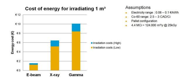
Efficiency illustration of the different radiation technologies (electron beam, X-ray, gamma rays)
