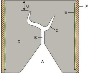
base of the casting ring and is made up of investment material. The crucible fromer can be made of rubber, wood, wax or other polymers.
