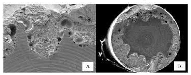
the casting ring (too great a thickness of the investment will resist the escape of air or gas from the mould)
